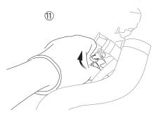
Follow the indicated direction to install the sensor and the adaptor to the original position.
