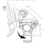
Follow the arrow direction to loosen the OEM sensor
