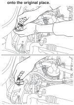
7.Set the adaptor and sensor. Then slightly press the adaptor down to get stuck with the intake manifold
