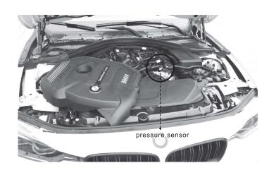
step2: Install the OEM pressure sensor on the adaptor
