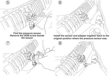
Install the OEM pressure sensor on the adapter.
