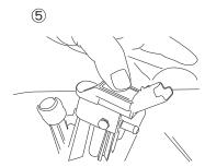
Install the sensor and adapter together back to the original position, amd press them down slightly to let them stick into the intake manifold a little bit.
