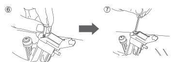
Take the attached screw and put it into the adaptor then twist it.
