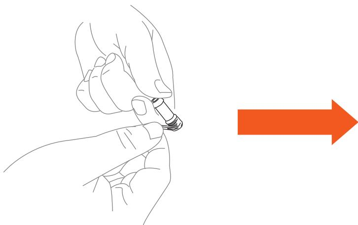
Apply Teflon tape or threadlocker to the aluminum pipe threads.
