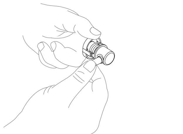
Tighten the adapter body clockwise; reinforce with tools if necessary.
