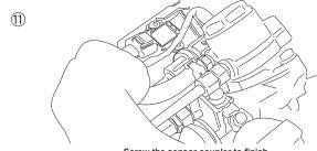
Screw the sensor coupler to finish.
