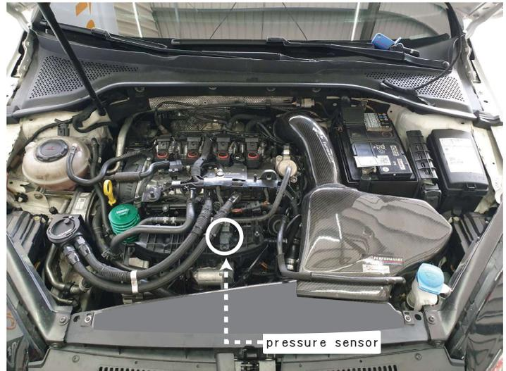
step2: Install the OEM pressure sensor on the adaptor
