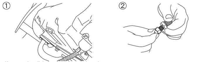
Unscrew the oil drain plug when replace the oil for maintenance
