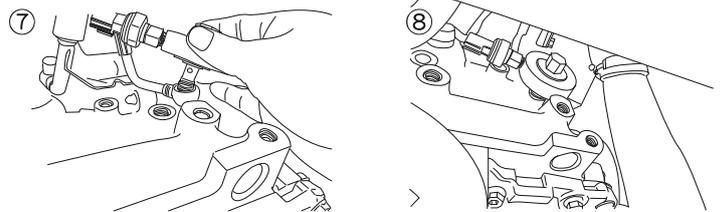
Screw the bolt into the oil return pipe.
