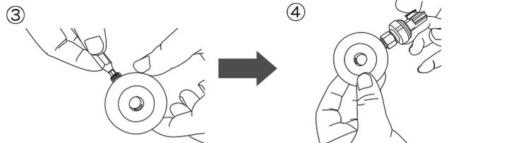
screw the 1/8" NPT nut into the VW CDL oil adaptor
