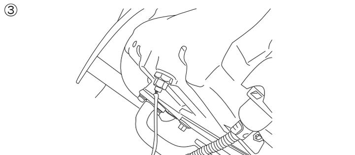
Screw the oil drain plug back to the oil return pipe.
