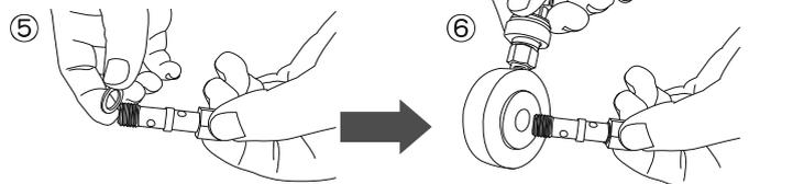
Fit the washer into the bolt for oil return pipe.
