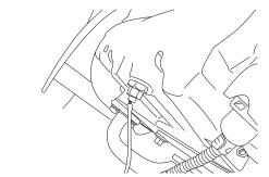
Screw the oil drain plug back to the oil return pipe.
