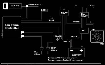
Installation by connecting the relay of ECU.
